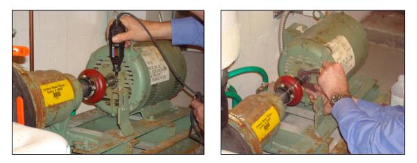
2) Epoxy the grounding ring onto the motor housing. The ring used at Blackstone was a Split Shaft Grounding Ring. This type is installed around the shaft, eliminating the need to remove the coupling which would require realigning the motor and pump.
