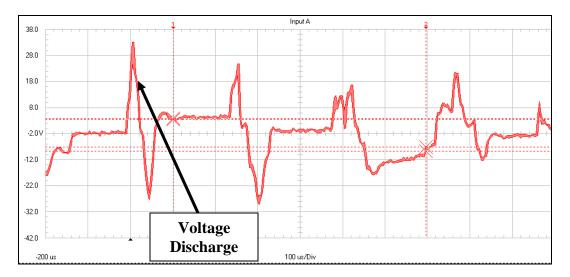
**Illustration #5: Test results from Motor #1 without a Shaft Grounding Ring.**
