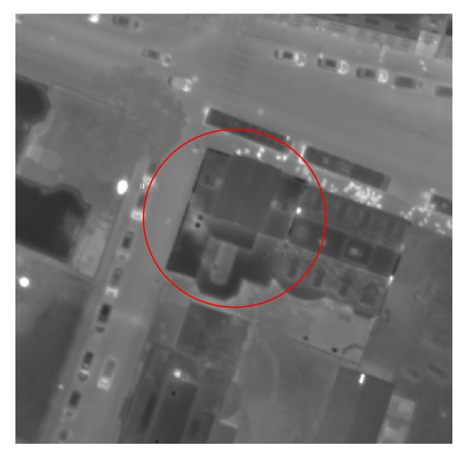
The above aerial thermographic image, taken during the winter months, shows MAS circled in red. White spots on the image are 'hot' areas where heat is being lost through the top of the structures.
