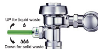
SLOAN UPPERCUT® Dual-Flush Flushometer (Up 1.1 gpf and Down 1.6 gpf)
