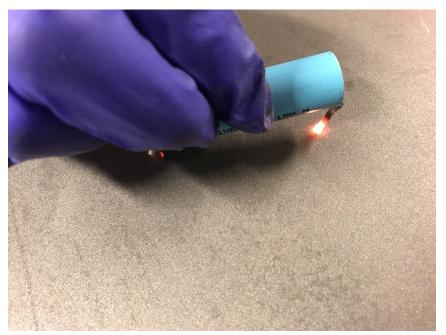
See attached photo showing how rechargeable batteries can spark and cause red-hot temperatures within one second of being touched to steel. We depend on you to keep our drivers, battery sorters, trucks and warehouse safe. Please spread the word to your occupants and residents.
