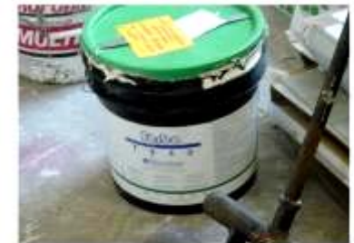
6/11/08 Low VOC Paints, Covered Containers
